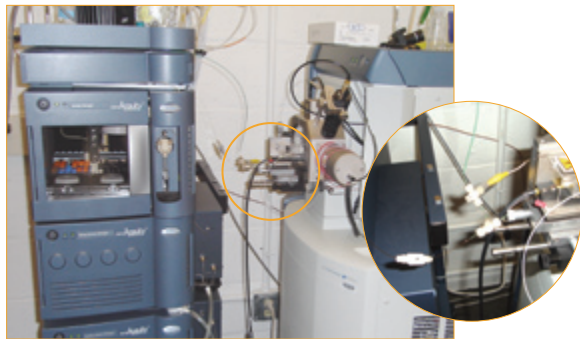
Figure 3 Waters nanoACQUITY UPLC™ System and Q-ToF Premier™ with PicoClear™ union, trap split (Upchurch® MicroTee), and liquid junction visible (inset). Pre-cut fused-silica capillaries insured clean mating of fittings, with easy confirmation of the trap column and union integrity.
