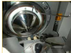
DPV-550 dual-column hardware, showing the positioning of columns relative to LTQ inlet
